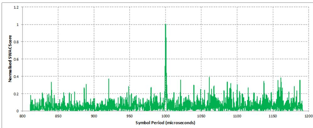
*SWAC detection of the GPS down-link signal in ATA data centered on 1575 MHz (signal entering through antenna side-lobes).*
