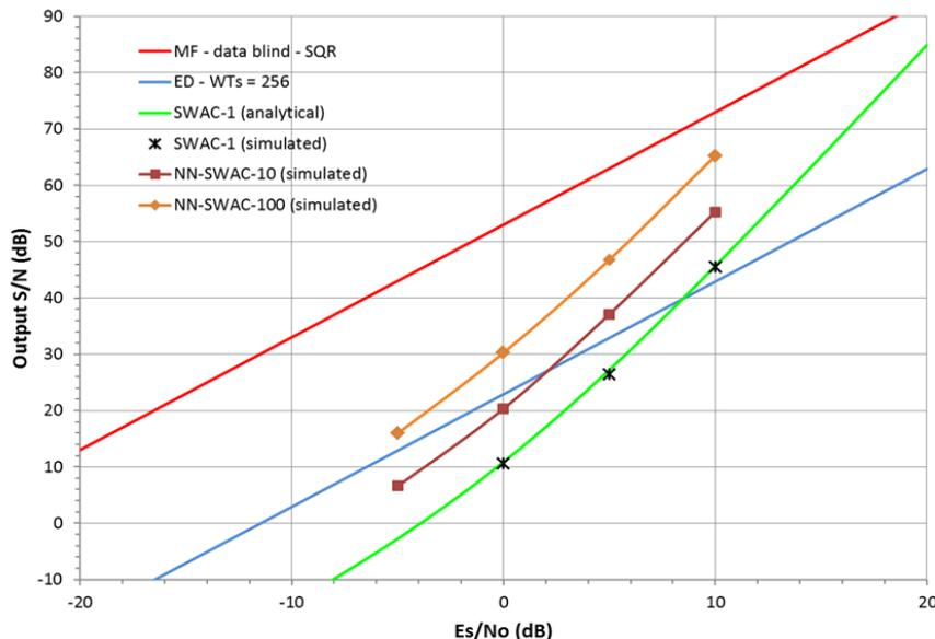
*Evaluation of SWAC sensitivity through simulation shows that advanced variants can outperform energy detection (blue curve) and approach the performance of matched filtering (red curve).*
